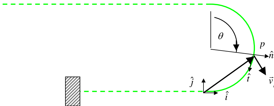
Figure 5. The velocity at point p is resolved into components along the local tangential and normal (\hat{t}, \hat{n}) .
