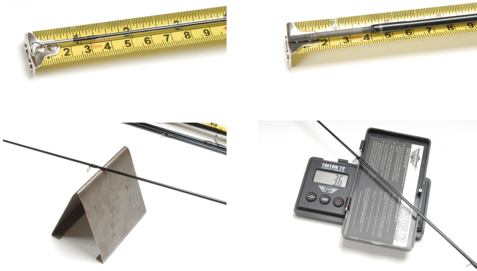
Figure 1: Pictures illustrating parts of the measure procedure. How the tip is measured, how spigot ferrules are treated, how the balance point (mass center) of a section is located and weighting of a rod section.
